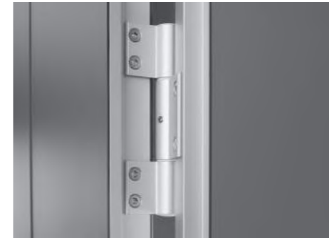
PRIMO Kn / PRIMO F: The three-roller edge hinge is durable, maintenance-free, screwed six-times and cannot be un-hinged.
